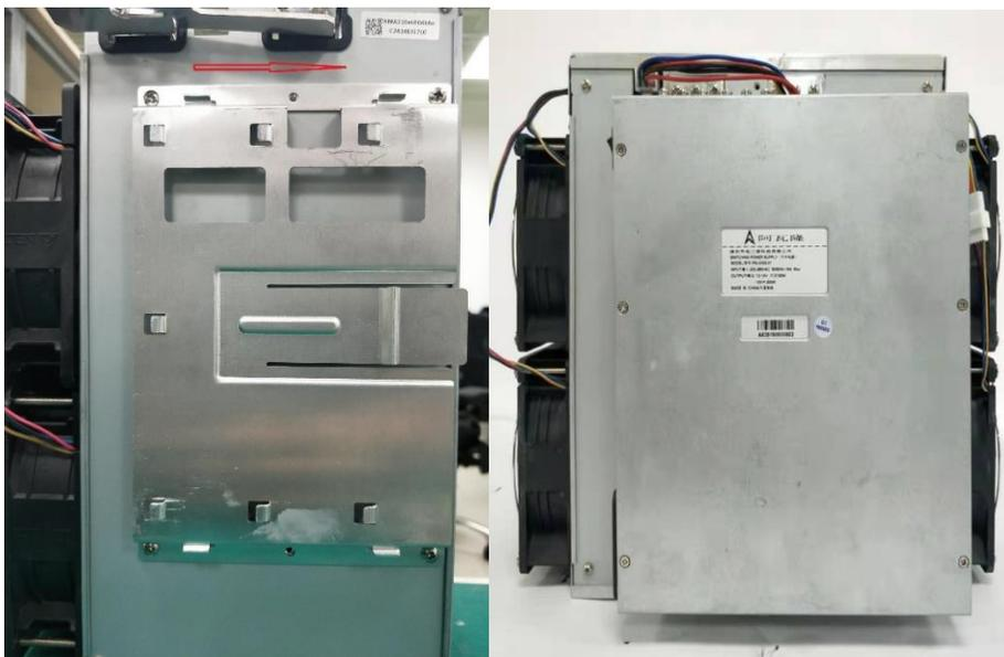
Please stretch the output copper wire to connect the PSU with the miner via 12 M4\*8 screws as the below Fig.
