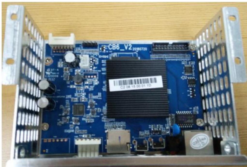
2) Insert the power control cable and the adapter board control cable into the corresponding slots on the control board, and then fix the bracket to the chassis with
