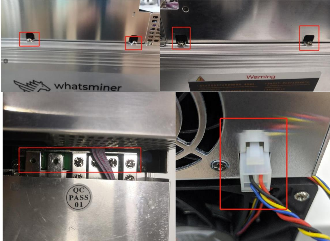
2) After the above operation is completed, gently pull out the power supply (do not pull out too long, the power control cable is still connected to the control panel), as shown in the figure:
