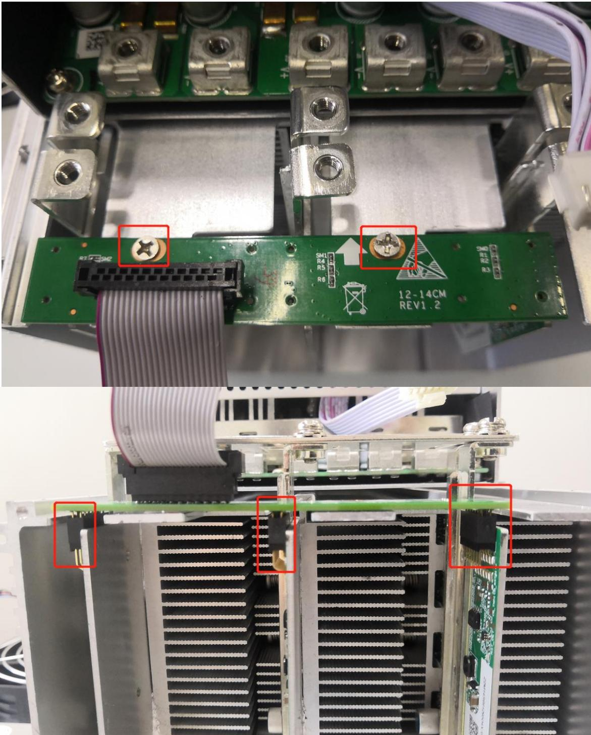
3) After the adapter plate is installed, install the copper bar. When the power busbar is connected to the hash board, the positive and negative poles of the copper bar cannot be connected incorrectly, and the screw pads of the fixed copper bar must be aligned with the edge of the copper bar, otherwise it may be possible to power on, and the machine will short-circuit. Fixed screws must be tightened to ensure the normal operation of the machine with proper contact with the copper bars, as shown:
