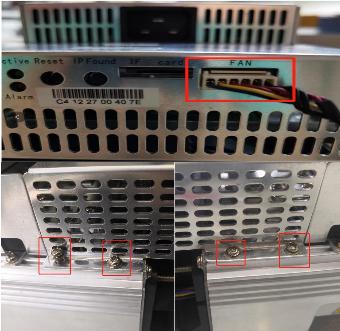
2) Unplug the power control cable and the adapter board control cable connected to the control panel as shown:
