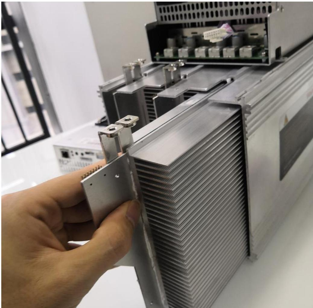
2) After installing the hash board into the chassis, first install the adapter board. **The**
