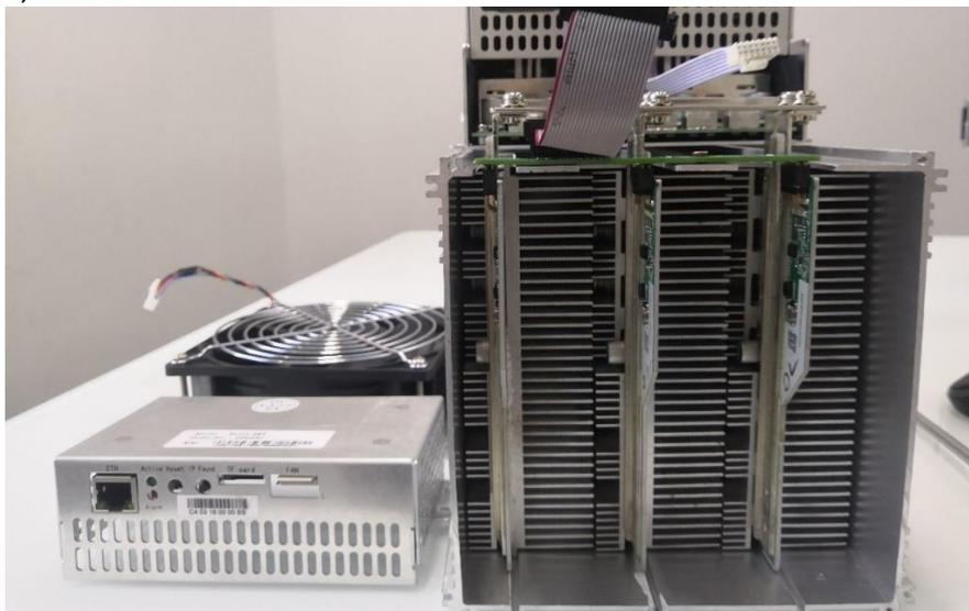
2) Remove the adapter plate and the copper bar fixed to the control panel as shown:
