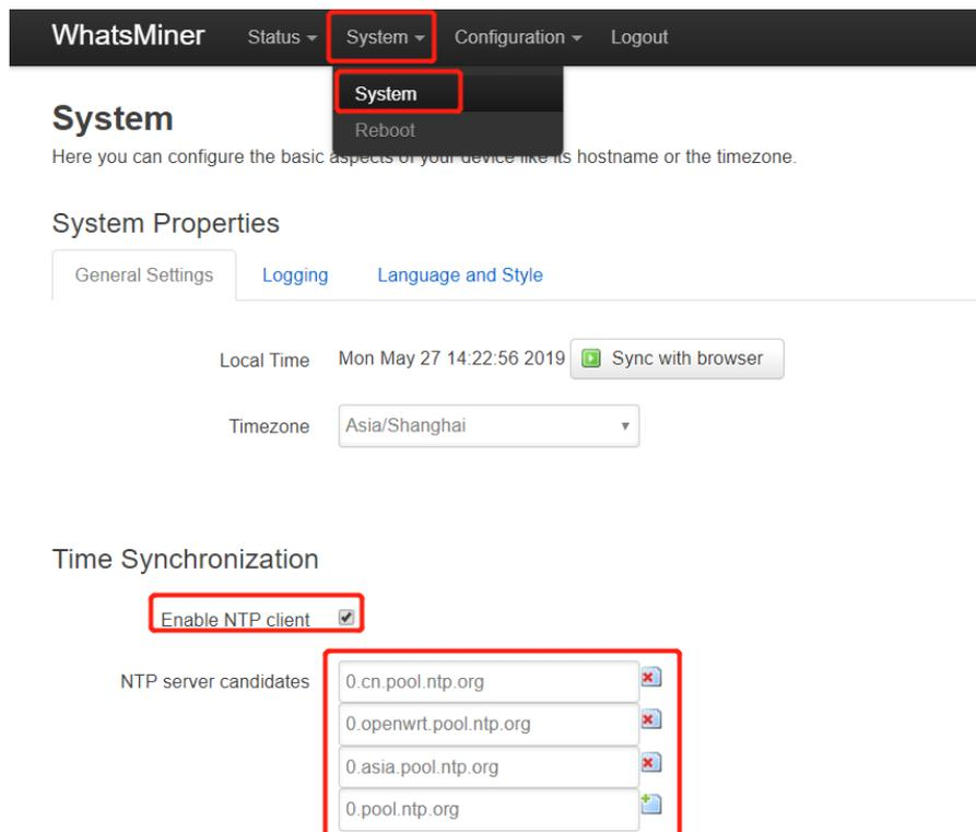
(2) In the CGMiner configuration interface, add or modify the NTP server address. The miner has been configured with four NTP server addresses by default. You can modify or add the NTP server address to the local NTP server address according to the mine situation.
