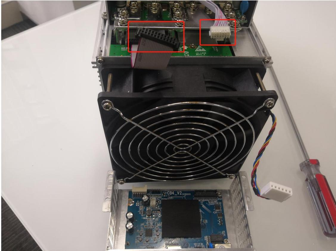
3) Remove the four screws fixed on the bracket and take out the control panel from the bracket as shown:
