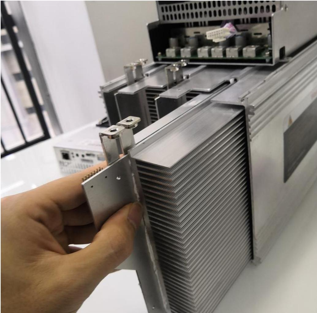
2) After installing the hash board into the chassis, first install the adapter board. **The socket of the adapter board and the pin of the hash board must be installed in place to avoid other contact related issues, as shown:**
