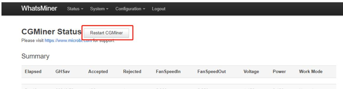
(4) Restart the control board and check whether the configuration modification takes effect. (If you do not choose to restart CGMiner, after the configuration is modified and saved, you can also restart the control board to make the configuration
