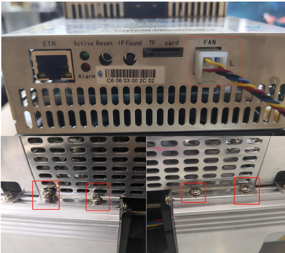
2) Unplug the power control cable and the adapter board control cable connected to the control panel as shown:
